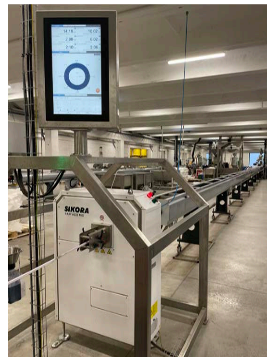
HÖHLE uses the X-RAY 6000 PRO for dimension measurement during the production of microducts
