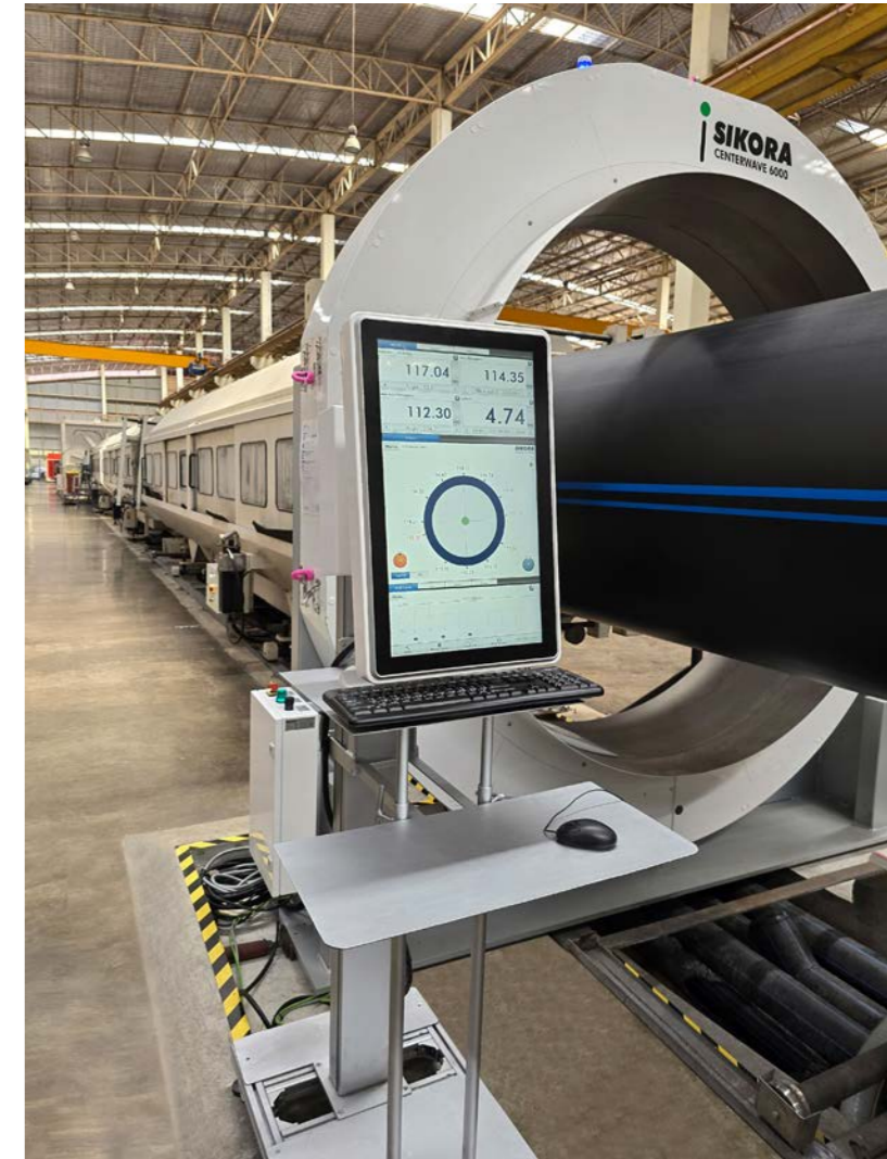
Thai-Asia P.E. Pipe uses the CENTERWAVE 6000 from SIKORA for continuous quality control of large pipes with wall thicknesses of more than 100 mm (3.937”).
