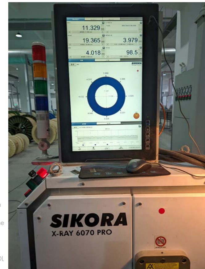
Wuxi Huacheng Cable uses SIKORA's X-RAY 6000 PRO for measuring and control during new energy cable production
