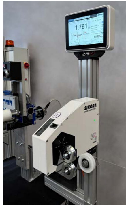
PMH GmbH uses the LASER LUMP 2000 from SIKORA for diameter measurement and detection of lumps and neckdowns.
