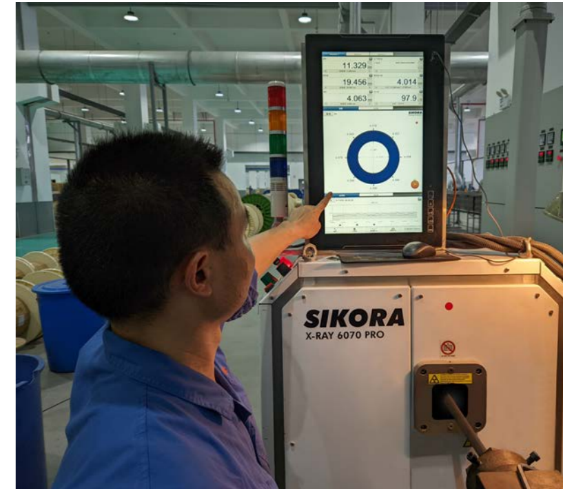
Wuxi Huacheng Cable uses SIKORA's X-RAY 6000 PRO for measuring and control during new energy cable production
