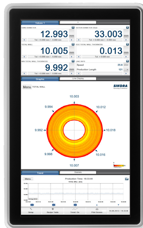
Monitor image: RF cable with foamed PE insulation
