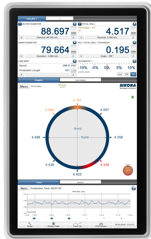
The production data of the X-RAY 6000 PRO is clearly displayed on the vertical 22" TFT monitor of the ECOCONTROL 6000
