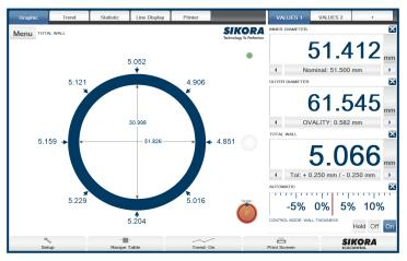
In addition to single-layer tubes and hoses, the total wall thickness of many multi-layer products can also be measured. In combination with the ECOCONTROL PURE, a processor system with a high-resolution 15" touchscreen display, the measured values are clearly displayed for further analysis. For measuring up to three layers, SIKORA also offers the X-RAY 6000 PRO.
