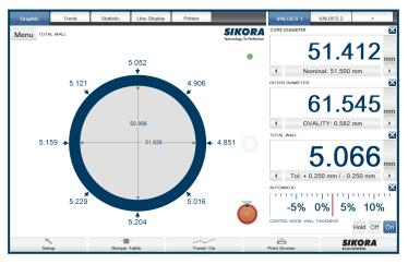
In addition to single-layer products, the total wall thickness of many multi-layer cables can also be measured. In combination with the ECOCONTROL PURE, a processor system with a high-resolution 15" touchscreen display, the measured values are clearly displayed for further analysis. For measuring up to three layers, SIKORA also offers the X-RAY 6000 PRO.
