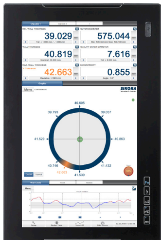
Measuring values of the CENTERWAVE 6000 at the ECOCONTROL 6000 processor system
