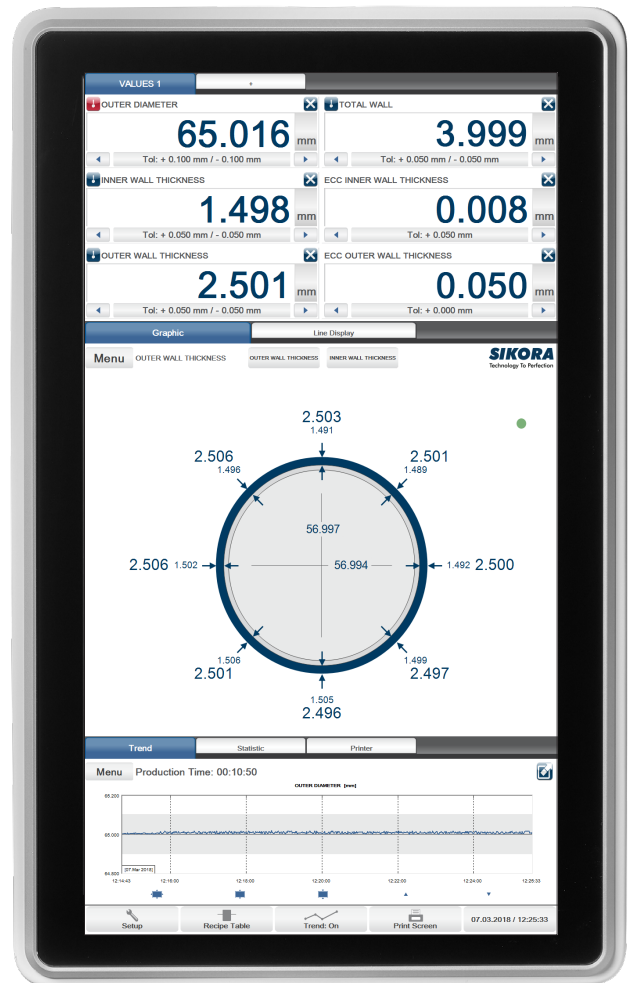
ECOCONTROL 6000: The production data of the X-RAY 6000 PRO is clearly visualized at the vertical 22" TFT monitor
