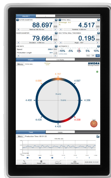
X-RAY 6000 PRO monitor image at the ECOCONTROL 6000
